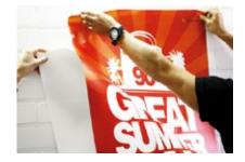
**3.** Remove the air between the film and the applied surface to assure strong adhesion. You can use the cardboard backer for this.
